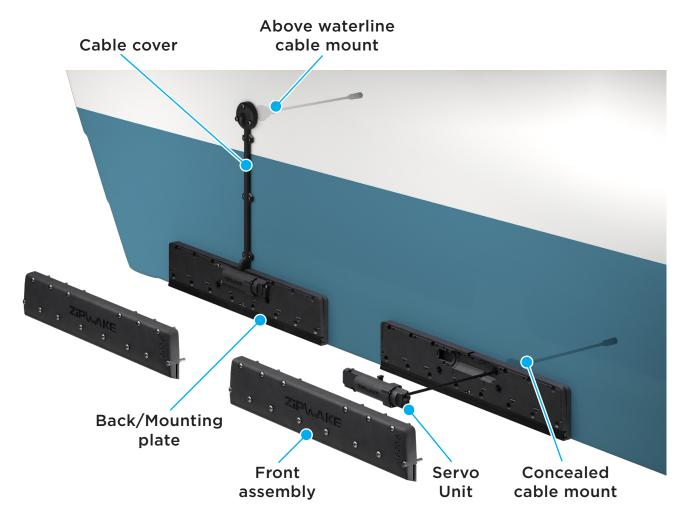
Different-sized interceptors can be favorably combined to span as much of the transom edge as possible. A full beam is always the optimal arrangement from a lift-to-drag ratio point of view.
