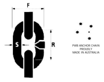
Abbreviations: S Dia F Width R Pitch MWL Max wkg load/tonne WWL Max mass which chain hanging vertical shall support in general service.
