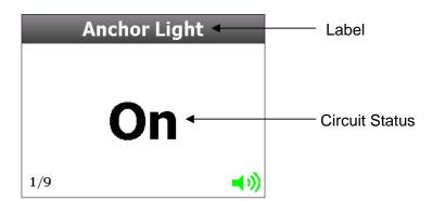
The systems in operation functions of this meter can be used to monitor essential circuits and inform the skipper about the circuit's state. Up to 8 inputs can be used as Systems Operation and they can all be displayed on the Mimic page for quick reference.
