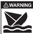
**Flood hazard. Before performing any service, close all waste system seacocks. Failure to do so can result in flooding which can cause loss of property and life.**
