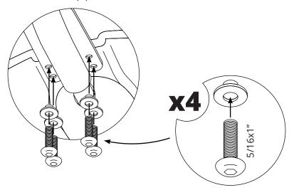
When using the Seaview #SP1-MOD or #SP2-MOD Spreader Kits use the 5/16x2-1/2" bolts.
