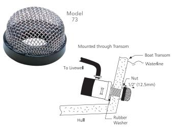
The Livewell Pump Debris Strainer attaches directly to any pickup tubes on Rule Livewell Pumps. Filters out trash and debris which could clog pump. Stainless steel wire mesh, 3/4" (19mm) female NPSM threads.
