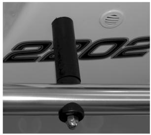
Complete the first standoff installation <u>using Loctite</u> tightening both the Acorn Nut and Backing Plate Nut.
