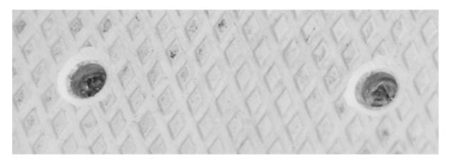
**Put 3M 5200 Adhesive in Holes and Base Location:** The 3M 5200 Marine Adhesive is a key structural part of any T-Top installation. Squirt 5200 into each hole and be sure it is filled with 5200. Then add a smooth layer about 1/16" thick between the four holes. The majority of the strength comes from the screws being bonded to the hole and the base being bonded to the deck adds additional strength. This should look like the image below.
